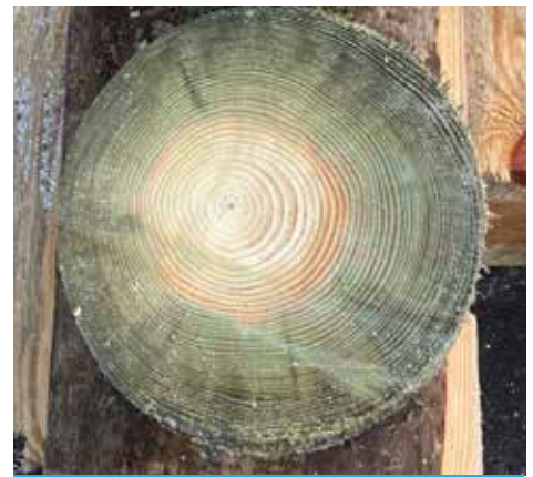
A cross-cut preservative treated post showing extent of formulation penetration.
